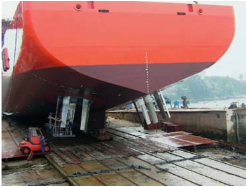
The two main Voith – Schneider propulsors are model VSP 36R6 EC/300; 3,800KW, @ 60rpm, electric driven, each weighing 100 tons with 6 x 2.8m long stainless blades..
