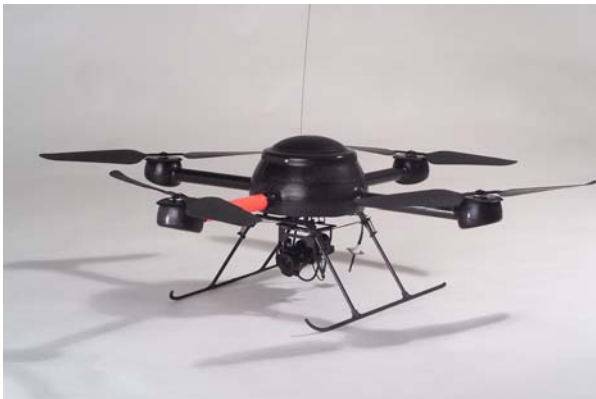
At sea the electric powered micro drone is always ready for instant take off, programmed to automatically search in a 600 meters wide zigzag pattern to 1.5km astern of the ship with its colour, tilt controlled video camera.
