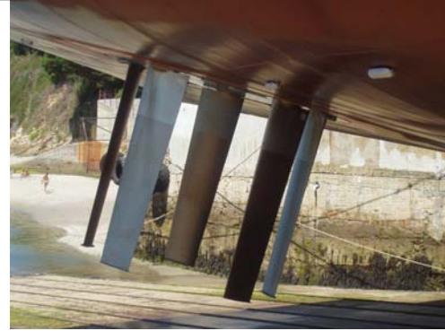
The two main Voith – Schneider propulsors are model VSP 36R6 EC/300; 3,800KW, @ 60rpm, electric driven, each weighing 100 tons with 6 x 2.8m long stainless blades..
